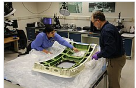
NTSB staff examine the door plug in the NTSB materials laboratory
