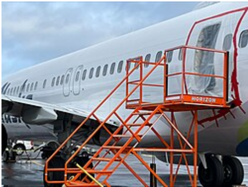
The aircraft, photographed on January 7, with plastic sheeting covering the missing door plug
